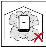
The inverter is designed to be dustproof in principle. However, in areas of high dust accumulation, the cooling surfaces can become dusty, which can impair the thermal performance. In this case, the dust must be removed regularly. We therefore recommend that installation is not carried out in areas and environments with high dust accumulation (e.g., iron filings) as this can cause damage to the inverter.
