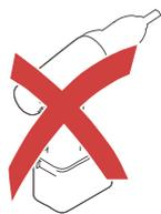
**Over torqueing with an electric drill will void the warranty**
